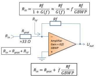
For AC signals the input resistance  $(R_{in})$  is increased by the virtual input impedance  $(R_{IV})$  of the I/V converter which is depended on the frequency (f), the feedback-resistor (Rf = gain) and the gain bandwidth product (GBWP) of the amplifier (see left). The *GBWP* of the *LNHS I/V Converter* is about 68 MHz.
