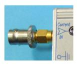
All the analog I/O signals are connected by SMA connectors to the device. If BNC connectors are preferred stable SMA/BNC-adapters can be screwed directly onto the *LNHS I/V Converter* (see left).
