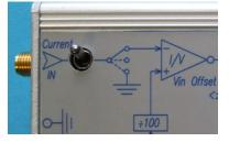
Grounding sensitive samples by using this input switch is strongly recommended during manipulations on the I/V converter (e.g. changing gain, power on/off).
