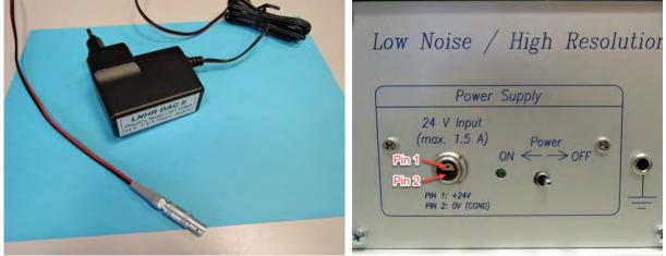
The LNHR DAC II can also be supplied from other clean 24 V<sub>DC</sub> sources, including batteries. The nominal 24 V<sub>DC</sub> voltage must be within a tolerance of  $\pm 10$  % and the device draws at maximum a current of 1.5 A<sub>DC</sub>. The needed power-plug is a 2-pin LEMO (type FFA.0S.302.CLAL44Z) with pin 1 connected to  $\pm 24$  V and pin 2 connected to 0 V.
