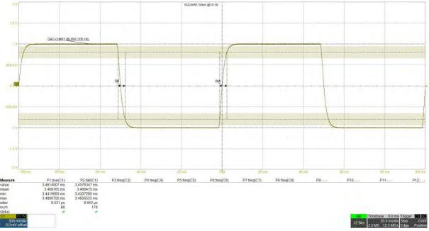
The measurement at LBW (100 Hz) shows no overshoot and a rise/fall-time of around 3.47 msec.
