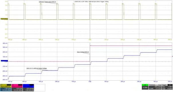
With each rising edge of the "Trig In AWG" input, the sinusoidal signal (predefined in AWG-A) is switched by one step. The time delay from the rising-edge of the external "Trig In AWG" input to the update of the DAC voltage is typical 6.3  $\mu$ sec and the time-jitter is about 1  $\mu$ sec.
