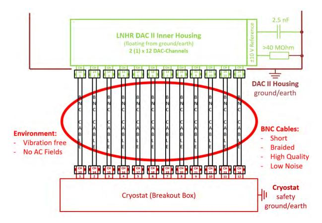
Wiring the DAC outputs to the cryostat should be done by using high quality and low vibration-noise coaxial BNC cables (e.g. Huber & Suhner G\_03130\_HT). The cable length should be as short as possible and they must be kept away from sources of mechanical vibration or electrical AC fields. Further, the coaxial cables should be braided together to minimize the open coupling area for AC stray magnetic fields.
