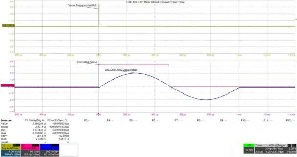
The minimum pulse-width of the "Trig In AWG" TTL input signal is 2  $\mu$ sec and the maximum repetition frequency is 40 kHz (every 25  $\mu$ sec).
