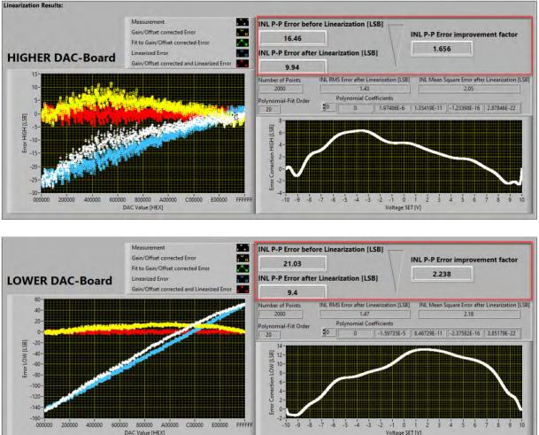
After the linearization procedure the residual "INL P-P Error" for both DAC-Channels are below 10 LSB which corresponds to an INL of only ±5 LSB. By applying this linearization process, the INL can typically be improved by a factor of two.
