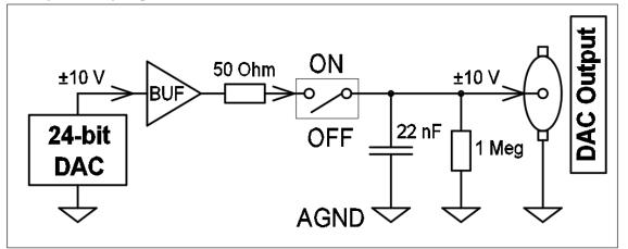
In the OFF state the output gets passively grounded (AGND) by a 1 Mega Ohm resistor in parallel with a 22 nF capacitor. The ON state is indicated on the front-panel by a LED next to the BNC connector; the color of the LED is depending on the selected bandwidth: Yellow = LBW (100 Hz) / Blue = HBW (100 kHz)
