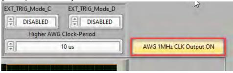
When time-synchronization has to be done, the AWG time-jitter can be reduced by switching to the "AWG Only" mode where the DAC-Board is exclusively working for the AWG function. Then all other DAC-Channels are blocked, and its last DAC voltages are frozen and they cannot be updated. The "AWG Only" mode can be set by a remote command or by using the "LNHR DAC II Commander" application (Tab 3 | AWG Control):
