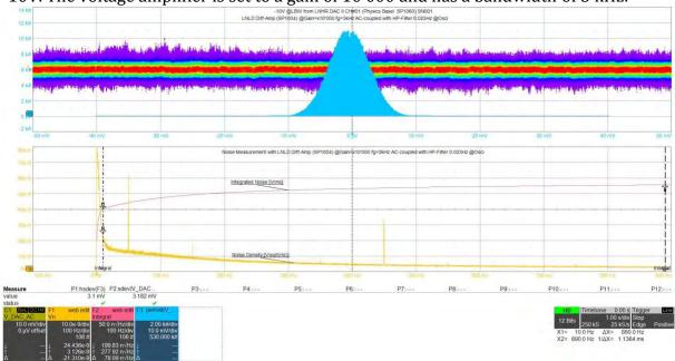
The top grid shows the time domain with 1 sec/div in the horizontal axis and 1  $\mu$ V/div (10 mV divided by 10'000) in the vertical axis; further the histogram (light blue) of 106 runs with 1  $\mu$ V/div (10 mV divided by 10'000) in the horizontal axis is shown. The accumulation of the 106 runs takes around 17 minutes.
