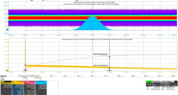
The top grid shows the time domain with 1 sec/div in the horizontal axis and 10  $\mu$ V/div (100 mV divided by 10'000) in the vertical axis; further the histogram (light blue) of 107 runs with 10  $\mu$ V/div (100 mV divided by 10'000) in the horizontal axis is shown. The accumulation of the 107 runs takes around 17 minutes.
