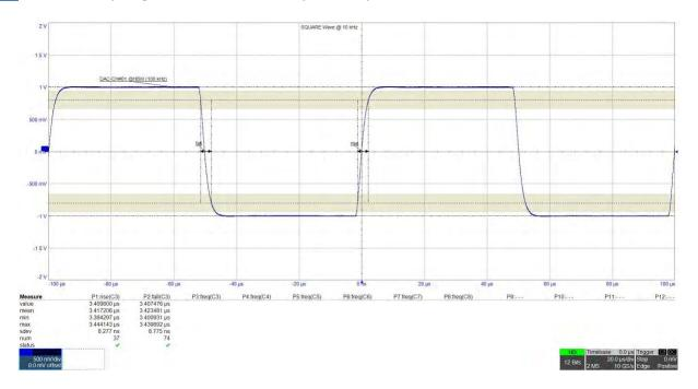
The measurement at HBW (100 kHz) shows no overshoot and a rise/fall-time of around  $3.42 \,\mu$ sec.
