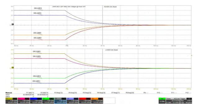
You can see that the eight DAC voltages decay smoothly (free from any glitches) to zero volts in the event of a blackout of the supply voltage. After about 100 msec the voltages have dropped zero. Therefore, even sensitive samples connected to the LNHR DAC II should not be damaged in the event of a power outage.
