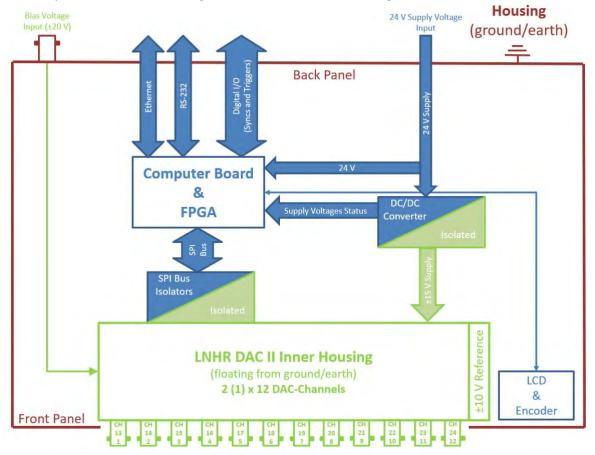
The shiels of the Ethernet cable, the RS-232 cable and the housing of D-Sub the connector for the Digital I/O are directly connected to the housing which is on ground/earth. Also, the reference-ground of the Digital I/O signals are internally connected to the housing (ground/earth). Because the sensitive DAC-Channels are well shielded and isolated from ground/earth, ground loops on these digital signals do not affect the low noise performance of DAC voltages.
