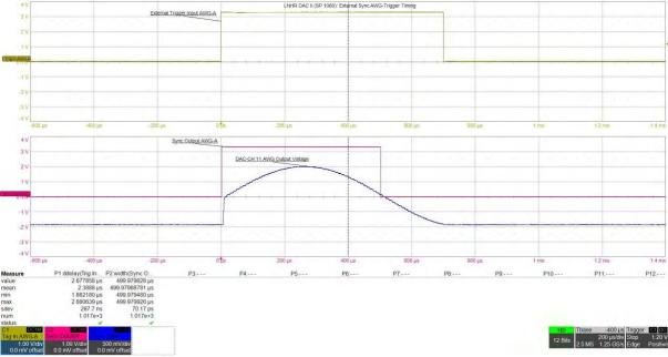
The rising-edge starts the AWG while the falling-edge stops the AWG after 700  $\mu$ sec. Since this is longer than the first half of the AGW-points the "Sync Out AWG-A" output signal has sill a pulse-width of 500  $\mu$ sec.
