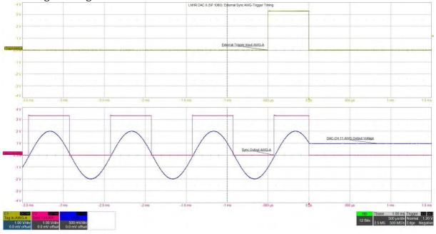
The falling-edge on the "Trig In AWG" input signal immediately stops the infinite repetitive running AWG. The rising-edge has no impact, since the AWG is already started.
